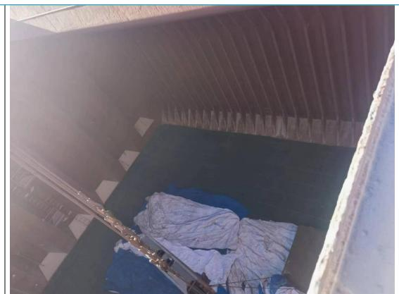
Before the loading process commenced, it was observed that within the cargo hold, another set of goods was arranged in a flat configuration and covered with a blackishgreen plastic woven cloth. To ensure segregation, a partition was established between these two batches of goods.
